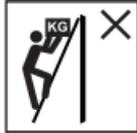
Do not carry equipment which is heavy or difficult to handle while using a ladder.
