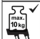
The multifunction tray or safety rail of the stepladder may be loaded with maximum 10 kg
