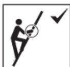
Keep a secure grip on the ladder when ascending and descending. Maintain a handhold whilst working from a ladder or take additional safety precautions if you cannot.
