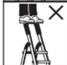
The multifunction tray or safety rail of the stepladder must not be used as a stepping surface.
