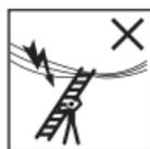
Use non-conductive ladders for unavoidable live electrical work.
