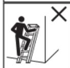
Standing ladders shall not be used as a leaning ladder unless it is designed to do so.
